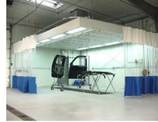
PAINT PREP BOOTH 14' x 24' can be customized to 18'-6" x 27' w/ 3' of circulation around booths
